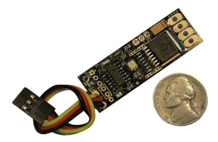
The Robot Power Wasp is a small low-cost high-performance single channel H-bridge speed controller for DC motors, and other electrical loads. The Wasp is designed for small combat robots, sumo robots, and other small robots such as firefighting robots, maze solvers and carpet rovers. The Wasp may also be used to drive pneumatic valves, solenoids, relays, thermoelectric coolers, and magnetic torque devices that require bi-directional control.
