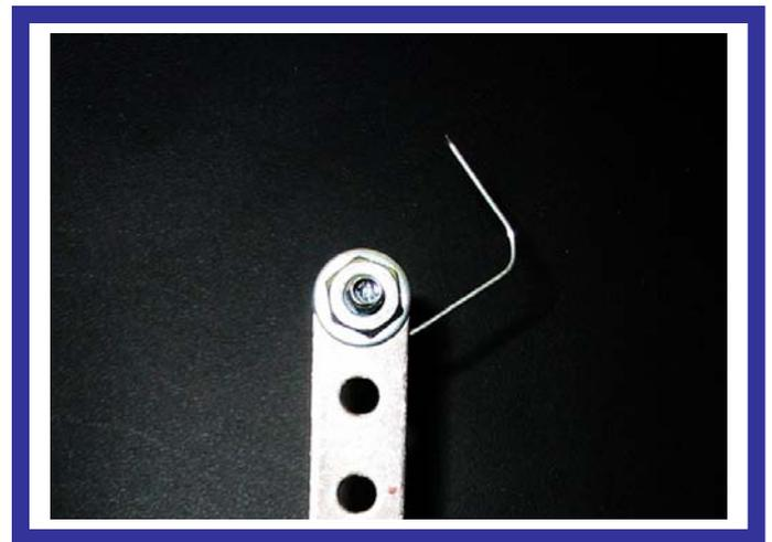
**CAUTION:** The slip hook is an important component of the trebuchet and it controls the angle at which the projectile is released from the throwing arm. The slip hook has a sharp end that can scratch your skin and lacerate an eye. Always wear safety glasses when working on, using or experimenting with a trebuchet.
