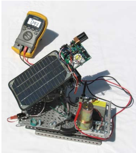
Figure 2-1: Board of Education Mounted on Solar Tracker Platform
