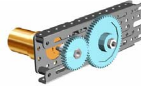
Fig 2.) Typical gear drive. In this example the drive ratio is 1.66:1
