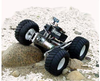
The HMC chassis can support over 200 lbs!
