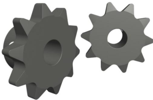
Fig.4.) 10 Tooth Solid Model w/ Bevel Tooth
