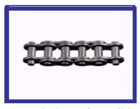
The #25 Pitch Plastic Chain included in the GEARS-IDS kits is made from Nylatron, a wear-resistant nylon filled with molybdenum disulfide (MDS). The tensile strength of the chain is approximately 75lbs.
