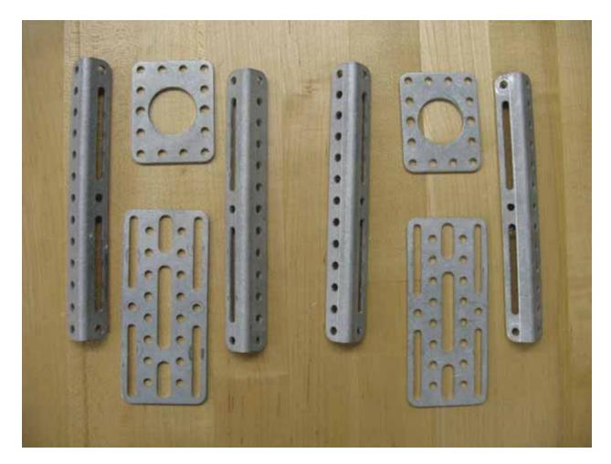
Take the 13 hole angles, the shaft plates, the M15 motor mounts, and line all the parts up as they are in the above picture. It is very important that you not only lay the parts out as in the above picture you need to build the side rail sub-assemblies so they are mirror images of each other. When the side rail sub-assemblies get mounted on the lower flat plate it is critical the parts line up from side to side.
