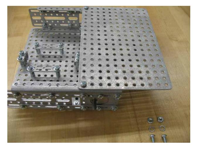
On the upper flat plate insert a 3/8" 10-24 bolt with a #10 internal star lock washer through the corner holes on each end of the left side. Then count 5 holes in on the side rail and insert the bolts through those holes as well. This bolt should line up with the left bolt in the M15 motor mount plate. With the bolts going through the upper flat plate and the side rail in the proper locations (shown above) thread a nut on the end of each bolt and lightly tighten the bolts up.
