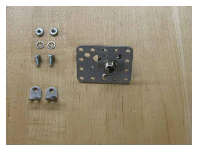
Take the "ON-OFF" plate and the mounting ring the off of the switch and insert the switch through the largest hole on the M13 motor mount. Now slide the "ON-OFF" plate back on the switch and screw the mounting ring down the switch to mount the switch on the motor mount. On the motor mount plate orient the switch so that the ON-OFF is facing side to side along the long side of the plate as shown above; make sure the switch is secured tightly.
