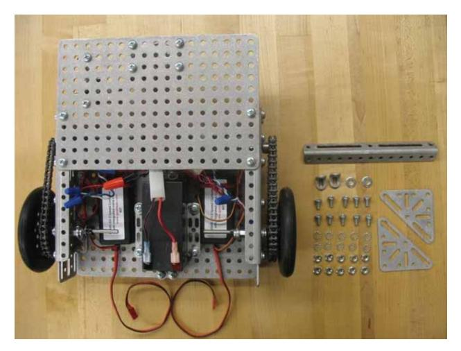
In this step you will be building the rear support bracket onto the Verminator Bot chassis.
