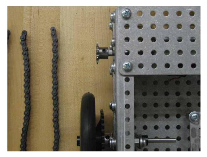
Slide the 10 tooth gear on to the shaft coming out of the gearhead motor. Make sure the 30 tooth gear on the wheel axle is tight against the wheel and the set screw is tightened up. With the 30 tooth sprocket in place line the 10 tooth sprocket up with the 30 tooth sprocket. Once the 10 tooth sprocket is lined up, tighten the set screw. Do this for both sides of the bot.
