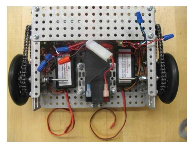
Connect the leads coming from the female end of the Molex wire harness to the corresponding terminals on the battery; black lead to the black terminal and the red lead to the red terminal. Then place the battery into the battery hold, with the battery in place you now can connect the male and
