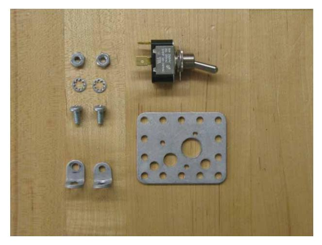
In this step you will build the switch mount sub-assembly.
