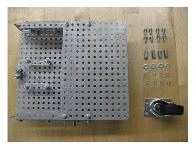
In this step you be installing the front wheel of the Verminator Bot.
