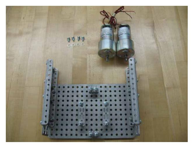
In this step you will be mounting two gear head motors into your Verminator Bot.
