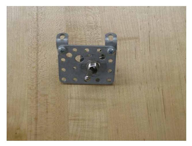
With the switch mount oriented as in the above picture install the 90 degree brackets with the slotted end facing away from the switch mounting bracket (shown above). Bolt the 90 degree brackets on the top row of holes on the switch bracket. Use the 3/8" 10-24 bolts, #10 internal star lock washers and 10-24 nuts to secure these 90 brackets. Only lightly tighten these as they may need adjusted to mount this sub-assembly to the bot.
