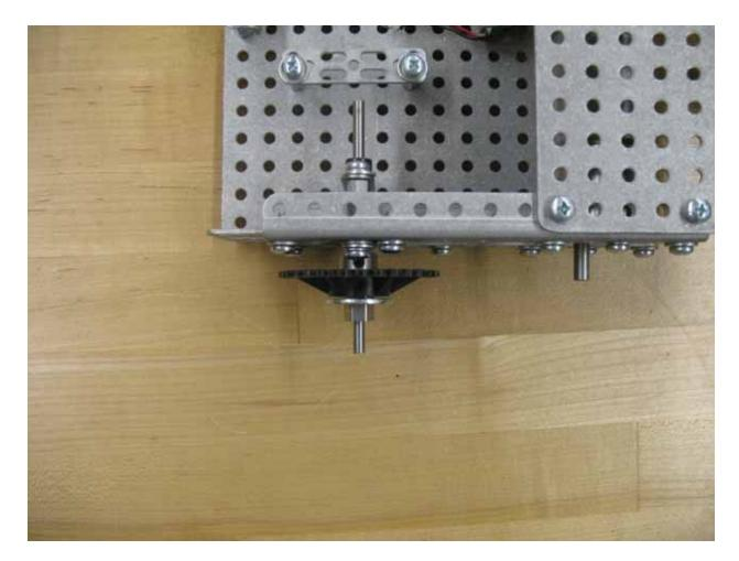
Slide the 30 tooth sprocket on to the hex adapter with the side that has the set screw in it facing out. Then slide a  $\frac{1}{2}$ " center diameter flat washer on the hex adapter as well. Do this for both axles on the bot. Do not tighten the set screws at this stage.
