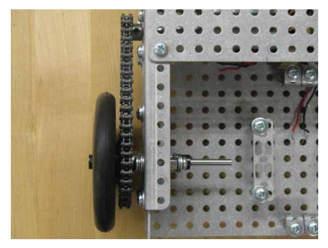
Slide the sprockets and chain back on to the bot, keeping the 10 tooth sprocket on the motor shaft. With the sprockets and chains in place slide the washers, wheel, and collar back onto the bot. Be sure to keep the 30 tooth sprocket tight to the inner side of the wheel. Once the 30 tooth sprocket is in position line the 10 tooth sprocket up with the 30 tooth sprocket and tighten it down. Turn the wheel by hand to feel for binding of any kind and adjust accordingly.
