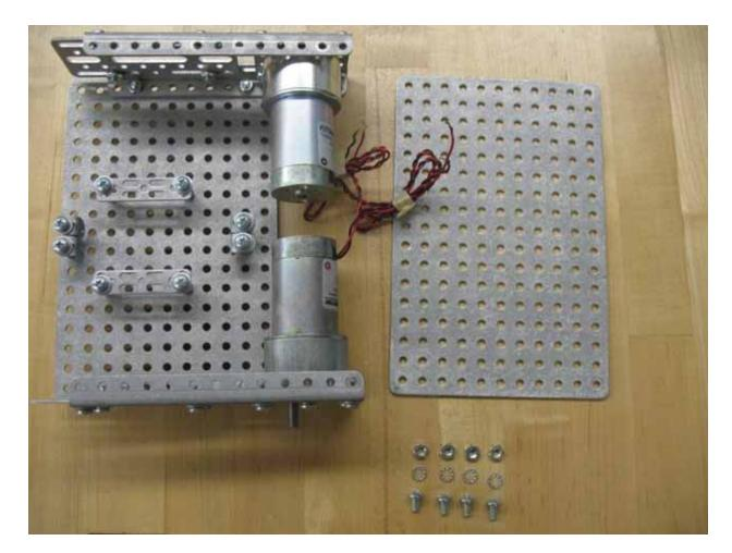
In this step you will mount the upper flat plate to the lower chassis subassembly.
