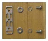
This is the proper order for placing the servo bracket, washer, lock washer, and bolt on the standoffs.
