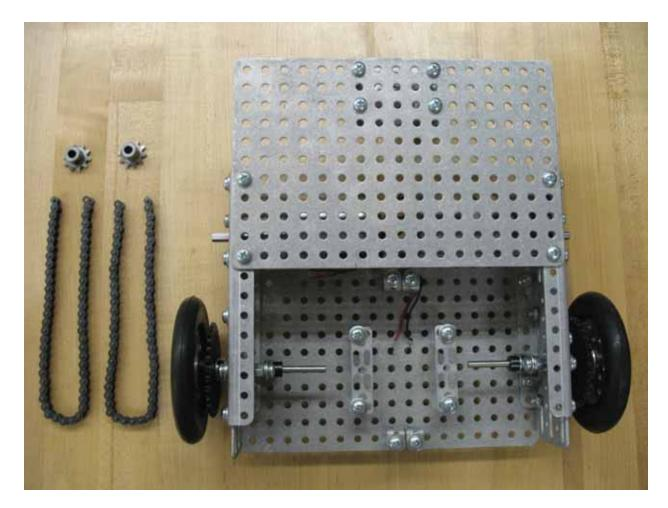
In this step you will be attaching the drive chains to the C.U.P. Bot.
