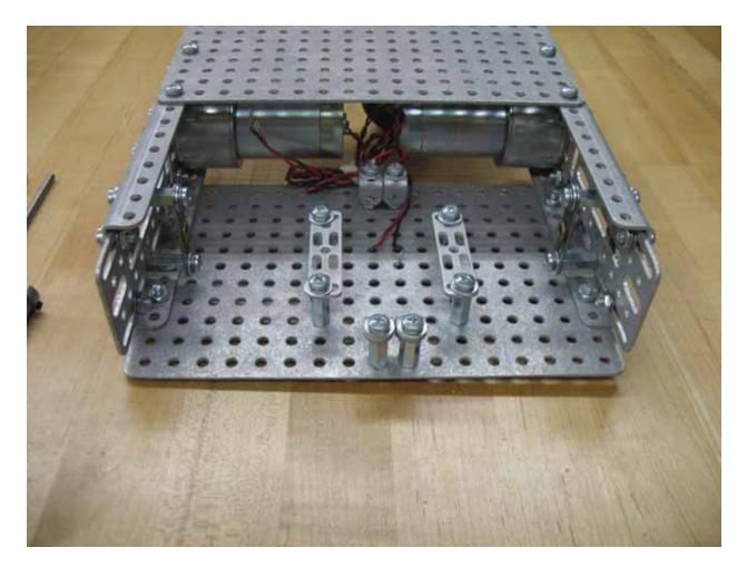
Install the inner bushing brackets by bolting them to the inner ends of the standoffs that are holding the outer bushing brackets on. Do this using ½" 10-24 bolts with #10 lock washers and flat washers. Put the lock washer by the head of the bolt and flat washer right behind the lock washer. Do this on all four bolts you use to install the inner bushing brackets. Lightly tighten these bolts as you did for the bolts that are holding the outer bushing brackets in place.
