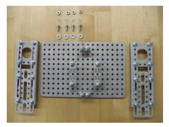
In this step you will build the lower chassis sub-assembly.
