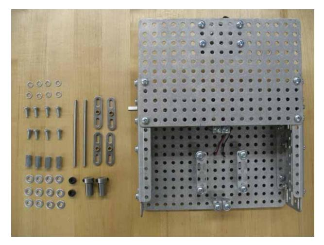
In this step you will be attaching the axles to the Verminator Bot chassis.
