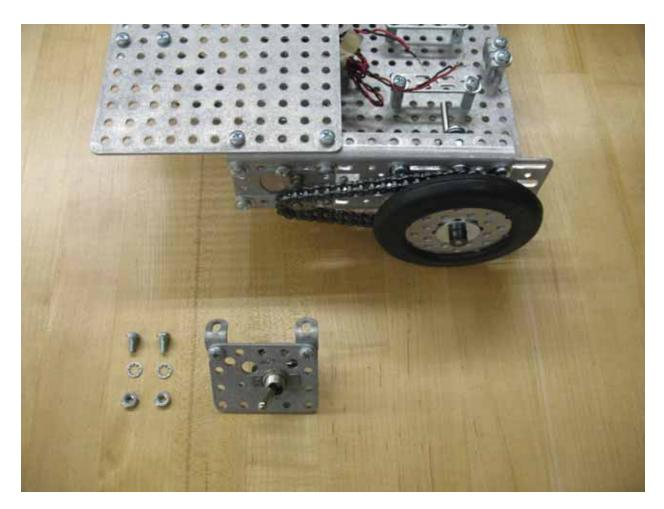
In this step you will be installing the switch mount sub assembly to the Verminator Bot.
