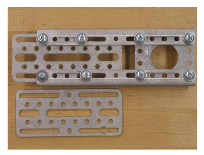
When attaching the shaft plate make sure the bolts going through the 13 hole angle go into the long openings on the top and bottom of the shaft plate. The shaft plate will be used to tension the drive chain on each side of the Verminator Bot later on in the assembly. So it is very important the shaft plate can slide forwards and backwards.
