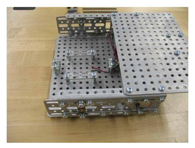
On the right side rail bolt a bushing bracket on using the same procedure from the last step. Keep the bushing brackets only lightly tightened as you will need to adjust these mounts when you adjust the chain tension. When you have both of the outside brackets installed your bot will look like the one pictured above.
