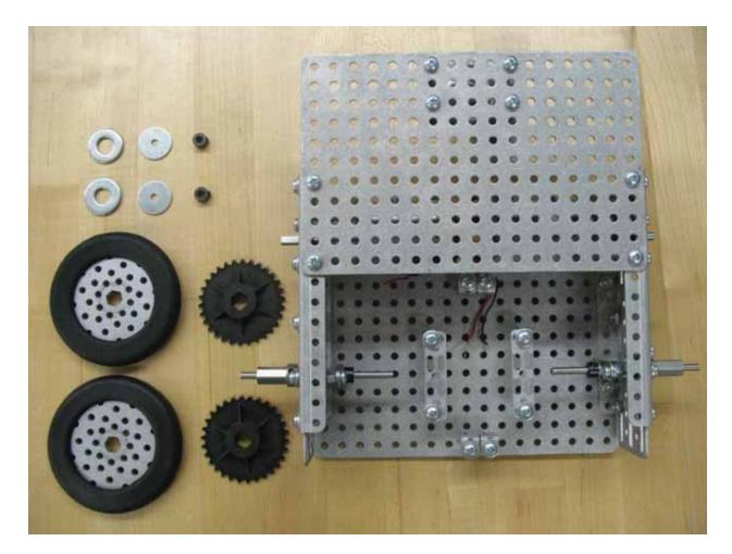
In this step you will be mounting the wheels on the axle shafts.
