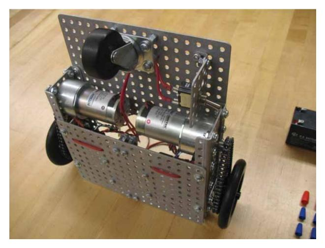
Take the two nine inch power wires and slide the female quick connector ends on to the male connector ends that are on the main power switch. Run the free ends of the wires around the standoffs that hold the swivel wheel on before running the wires to the back of the bot. This will help keep the power wires from interfering with the movement of the swivel caster.
