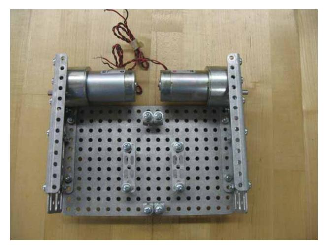
When both of your gearhead motors are mounted, their output shafts will line up from one side of the Verminator Bot to the other with the output shafts being oriented close to the shaft plates on the side of the bot. If they do not line up or are oriented so the output shafts are far from the shaft plates you need to remount one or both of the motors so they are oriented on the bot correctly.
