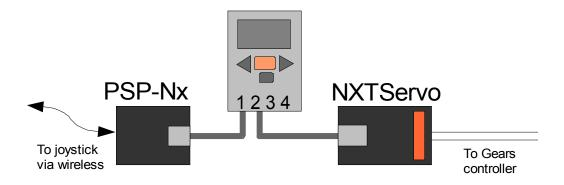
Picture below shows the electrical connections between Gears controller and NXTServo pins. Connect left Gears controller to SV1 and right controller to SV2.
