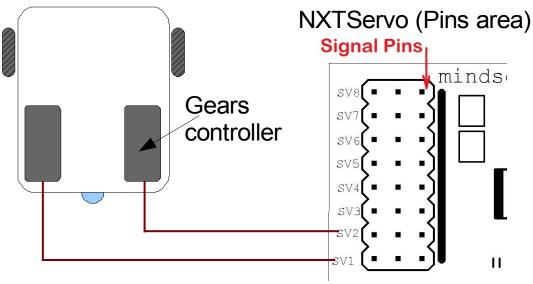
Ensure that the signal pin of Gears controller matches with the signal pin shown above.
