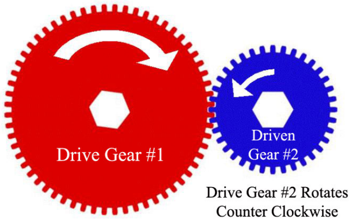
Fig. 6.3.1.7a Rotation of Two Gear Drive
